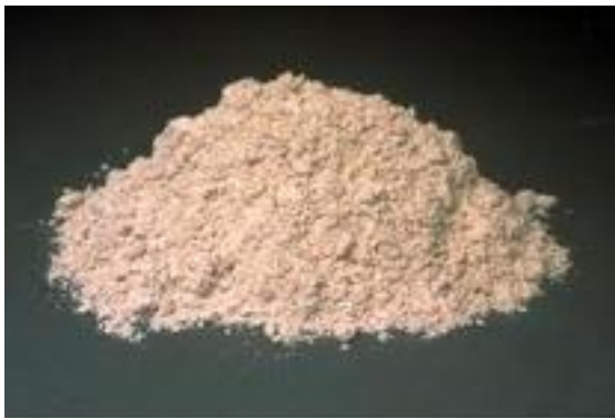
Figure 1 Slag Cement (ground granulated blast furnace slag)
