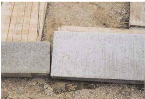
Figure 1: IS blended cement (33% slag content) was used to produce a noticeably lighter concrete masonry unit on the right
