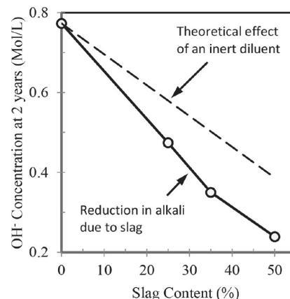
Figure 3: Effect of slag on pore solution alkalinity.
