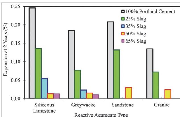
Figure 2: Effect of slag on the expansion of concrete containing reactive aggregate. Max limit of 0.04%.
