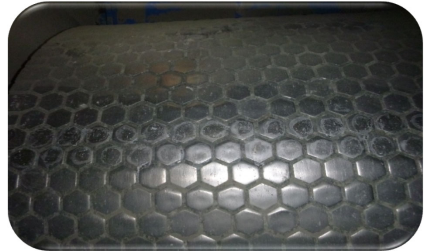
After 22000 hours, wear rate 1,5 to 1,8 mm per 10000 hours of operation
