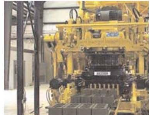
Concrete block machine producing block with slag cement.
