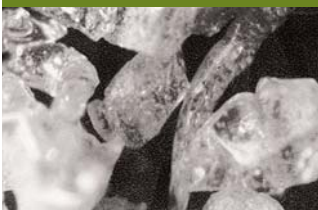
Microscopic slag cement illustrating its glassy nature
