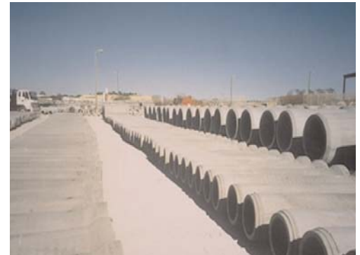
Stockpiled concrete pipe, manufactured with slag cement.
