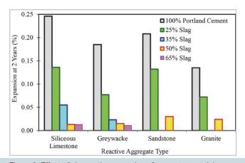
Figure 2: Effect of slag on the expansion of concrete containing reactive aggregate. Max limit of 0.04%.
